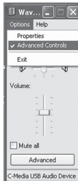
8. Click the "Advanced" button to open the "Advanced Controls for Wave In" window. Depending upon your system, you might have the option of selecting "1 AGC" or "Mic boost". Checking this option will significantly increase the sensitivity of the microphone. Use this for recording softer sounds. If you experience distortion when recording louder sounds, try unchecking this option.
